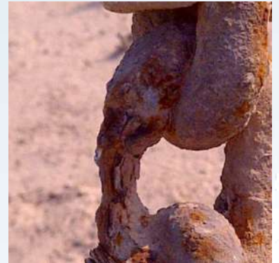
Rust on main halyard chains
